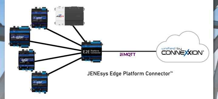
The JENEsys Edge Platform Connector is equipped to consolidate traffic of multiple Niagara instances in the same building and allows for a single point of exit for multiple devices. For example: a building with ten Edge devices could all point to one platform connector to route data to Connexxion.
