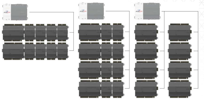
Each JENE-PC8000-R-34 can power up to (4) JENE-PC8000-R-16 Each JENE PC8000 is capable of supporting 250+ data points
