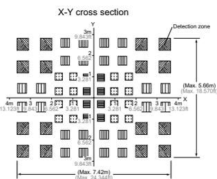
1. The X-Y cross-sectional diagram shows the detection area.
